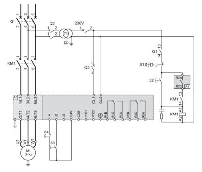
With Line Contactor, Freewheel or Controlled Stop
